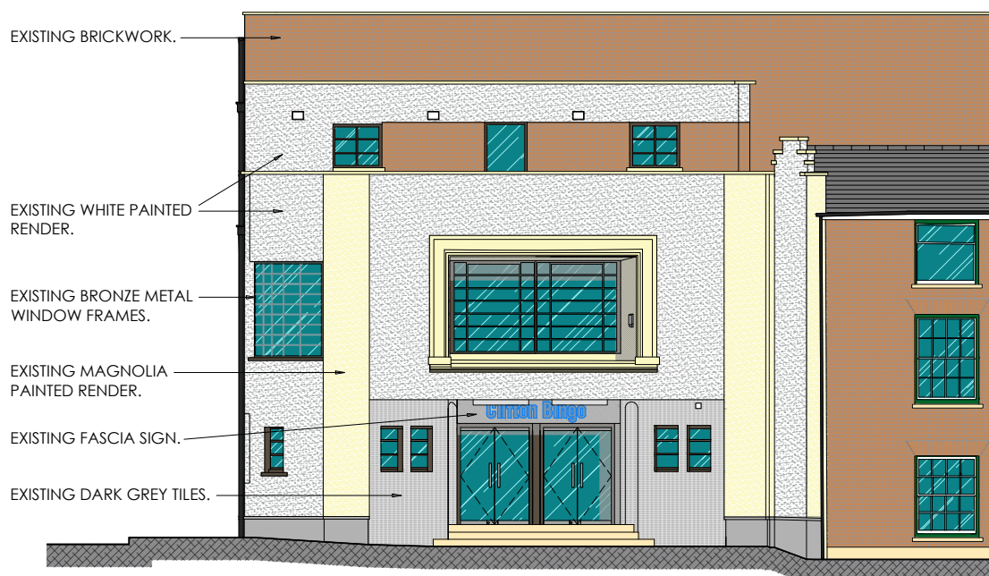
PROPOSED ELEVATION FROM SOUTH STREET, SHOWING THE RETENTION OF THE EXISTING FAÇADE
