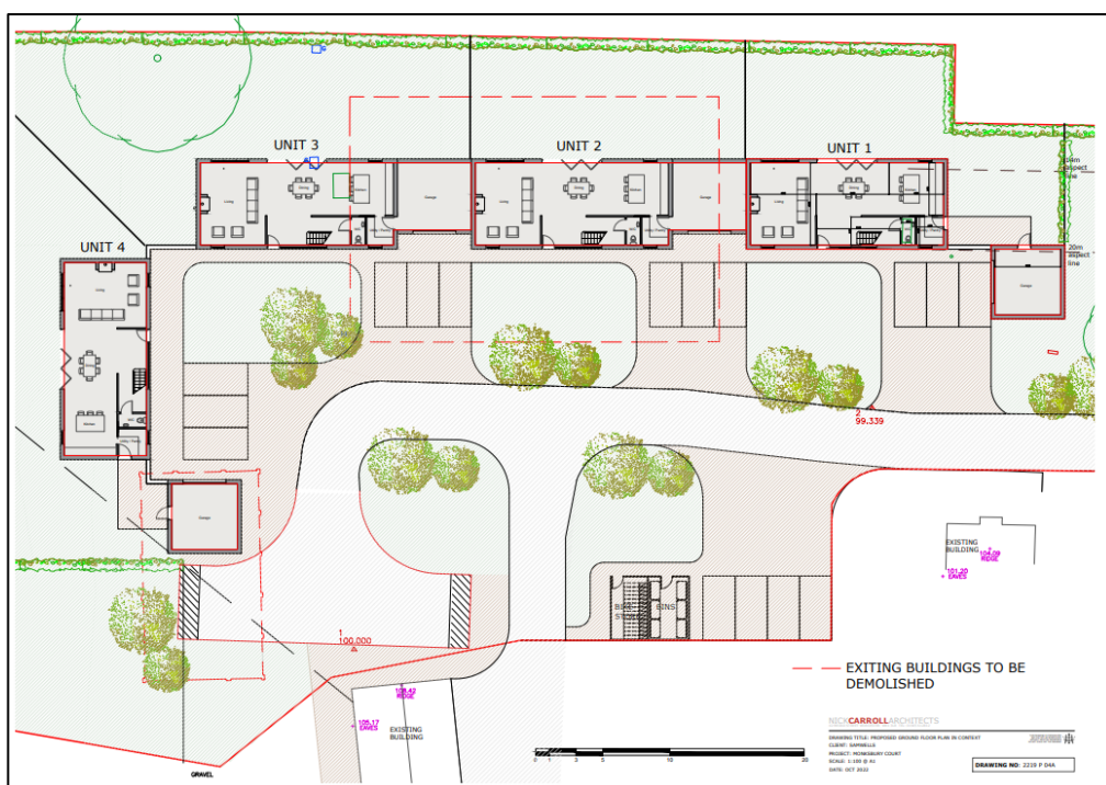
Figure 2. Proposed ground floor plan in context (Drg Number 2219 P 04A)
